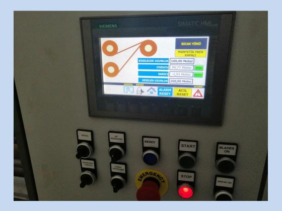
On the control panel, one would find controls of main motor speed, top and bottom coiling torque and brake power. There's an AC motor driver, and drivers for brakes, servo drivers for coils that provide individual winding and unwinding manually. An electronic encoder measures the length of the slit material length to keep track of how much the machine has slitten the material that is placed on the shafts.
